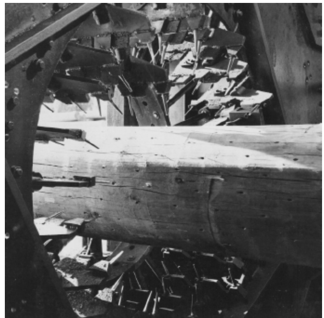
Figure 14-2. Deep incising permits better penetration of preservative.
