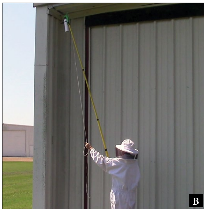
Figure 12. This Gotcha Sprayer is connected to a telescoping pole that allows application of aerosol insecticides to honey bees nesting overhead without climbing a ladder. The applicator pulls the twine, and the hinged, green lever depresses the top of the sprayer canister to release the insecticide. (Photo by J. W. Harris)
