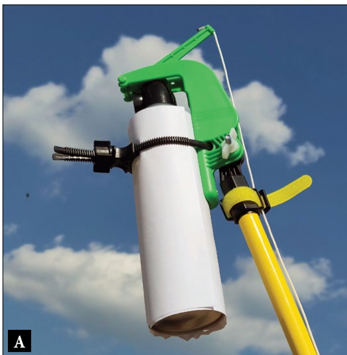
Figure 12. This Gotcha Sprayer is connected to a telescoping pole that allows application of aerosol insecticides to honey bees nesting overhead without climbing a ladder. The applicator pulls the twine, and the hinged, green lever depresses the top of the sprayer canister to release the insecticide. (Photo by J. W. Harris)
